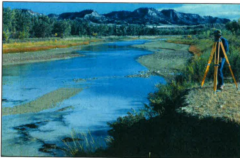
PR130. Top. 18 August 1986. View is downriver along the right bank, showing the new sand (0.1-0.3 m) on the point bar. J. Moody (~1.9 m tall) is standing at station 72. Bottom. 19 September 1988. View is upriver. J. Moody and tripod with level are just upriver from section PR130.
