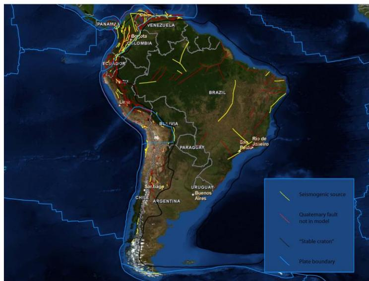
Figure 4. Crustal faults applied in hazard model.
